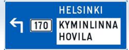
F11: Advance direction sign (above the lane)
