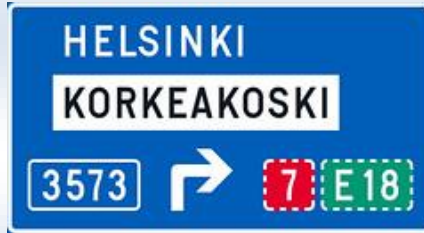
F10: Advance direction sign (above the lane)
