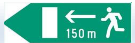
F57.1: Direction of emergency exit
